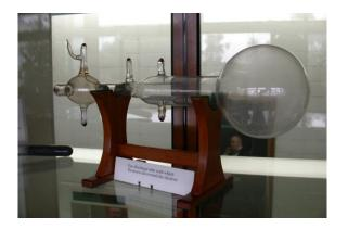
Principle : Electron beam deflected by central electrode
