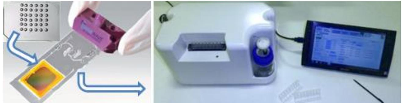
Modular system for multi-parametric optical detection using an automatised biological protocol. First validation by detection of several microtoxins
