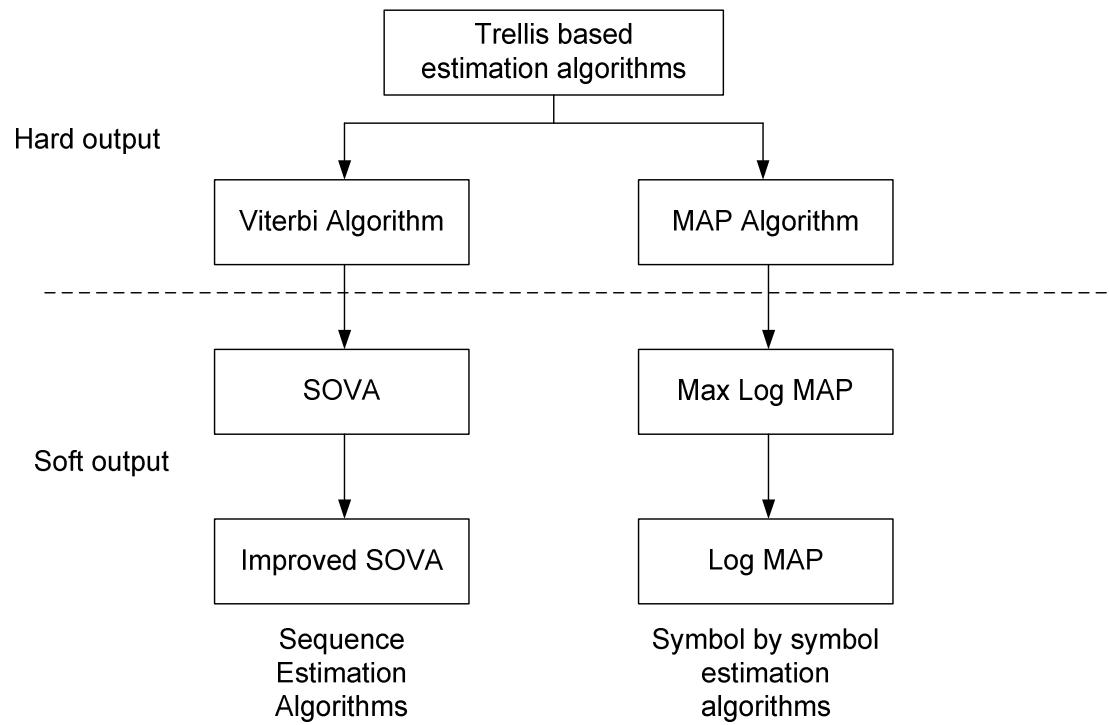
$$\begin{aligned}\max^*(x, y) &= \ln(e^x + e^y) = \\ \max(x, y) + \ln(1 + e^{-|y-x|}) &\approx \max(x, y).\end{aligned}$$
