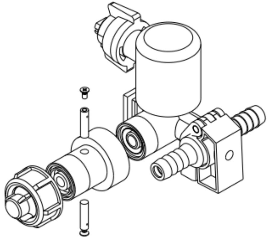
**Details of the smart sensor customized to measure the response time of a system of direct injection of pesticides.**
