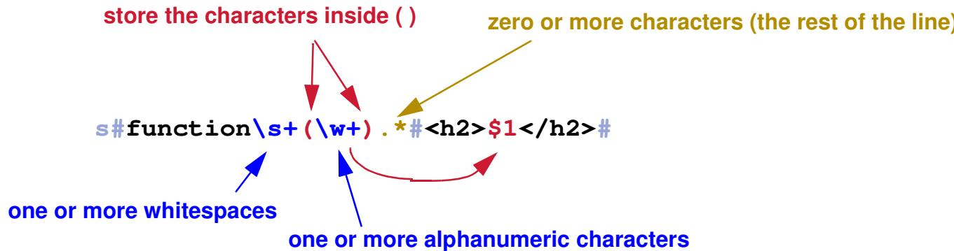
The diagram shows the perl-syntax pattern substitution command with annotations:
