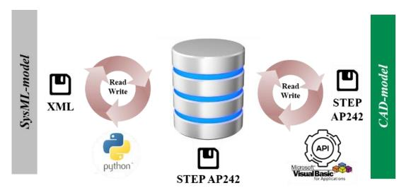
Interface concept, to link SysML- and CAD-models
