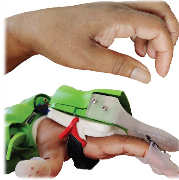
Image showing a stroke survivor's hand with hyperflexion in the fingers being offset by WiGlove.
