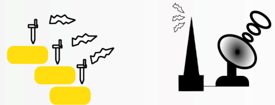
Ground communication network is formed by probes installed in the silos, a hub (data concentrator) coupled to a ground station that transmits the signal to the satellite.
