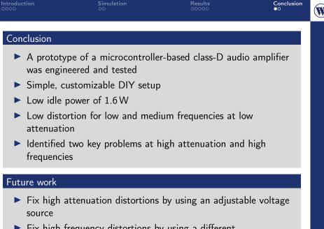
Fix high frequency distortions by using a different microcontroller (e.g., STM32WB55)
