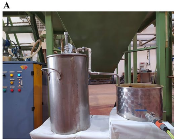
Fig. 1. Pilot plant for EO extraction. A) Steam distillation pilot plant B) EO and hydrolate detail.
