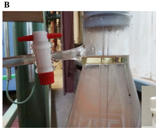
Fig. 1. Pilot plant for EO extraction. A) Steam distillation pilot plant B) EO and hydrolate detail.
